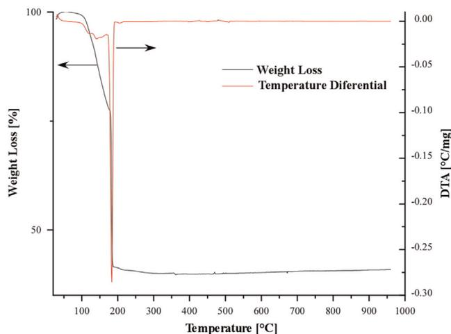
**Fig. 1.** Thermogram of the  $\text{Nd}_{0.05}\text{Bi}_{0.95}\text{Fe}_{0.95}\text{Co}_{0.05}\text{O}_3$  precursor powder prepared via combustion method at 250 °C.
