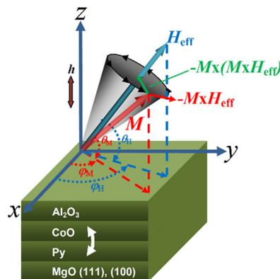
Fig. 1. Relative orientations of the external magnetic field (*H*) and magnetization vectors (*M*), the used coordinate system and picture of the prepared bilayer structure.
