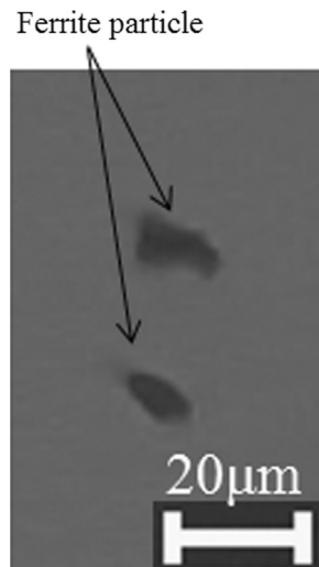
Fig. 1. Typical microscopy image of ferrite particles.
