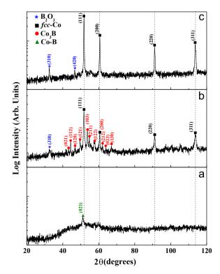
**Fig. 1.** Comparison of the XRD plots for the as-prepared, 250 °C and 500 °C annealed samples. The intensity is normalized to the same incident intensity for all the samples, and the scale is set accordingly.
