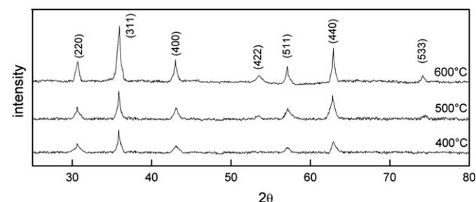
**Fig. 1.** X-ray diffraction patterns of MgFe<sub>2</sub>O<sub>4</sub> thin films calcinated at different temperatures.
