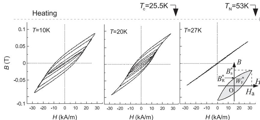
Fig. 1.  $B$ – $H$  loops with various field amplitudes  $H_a$ , taken at different temperatures on heating; 10 K and 20 K below  $T_c$  and 27 K above  $T_c$ . The inset shows the parameters of a  $B$ – $H$  loop;  $B_a^*$ ,  $B_R^*$ , and  $W_F^*$  are the maximum flux density, remanent flux density, and hysteresis loss, respectively.
