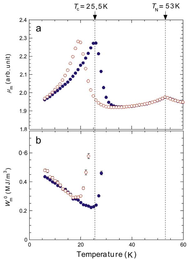
Fig. 2. (a) Minor-loop initial permeability  $\mu_m$  and (b) coefficient of a scaling power law,  $W_m^0$  as a function of temperature. The solid and open circles represent the data taken on heating and cooling, respectively.
