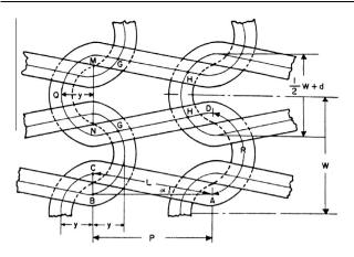
Figure 1 Loop shape of jersey knitted fabric by Benltoufa et al. [22].
