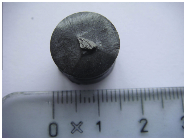
Fig. 1. The top view of the as-grown YBCO bulk prepared by TSMTG process in air.
