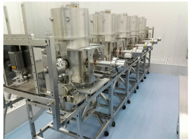
Fig. 4. Cold mass assembly in a clean room.
