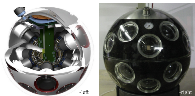
Fig. 1. Technical drawing (left) and assembled DOM (right) of the KM3NeT show the geometrical configuration and distribution of the several PMT [18].
