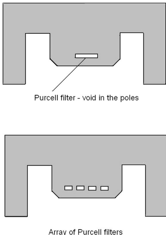
Fig. 1. Purcell filters used for improving field uniformity — single slot and an array of slots. Only half of the magnet is shown in two dimensions.
