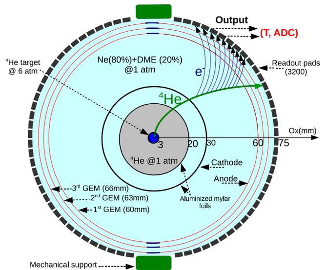
Fig. 2. Schematic drawing of the CLAS RTPC in a plane perpendicular to the beam direction. See text for description of the elements.
