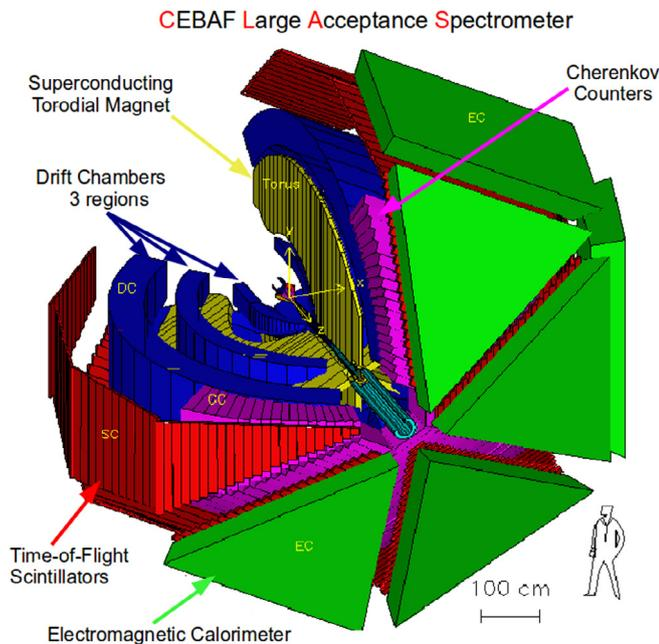
Fig. 1. A three dimensional representation of the baseline CLAS setup. The full description is given in the text.
