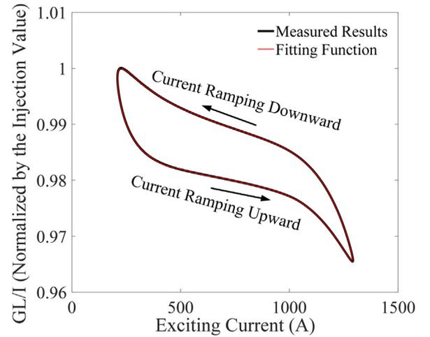
**Fig. 2.** The measured results of the relation of  $I - GL$  and the fitting functions.**Table 2**
