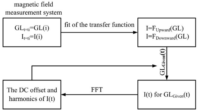
**Fig. 1.** The flow process diagram for the wave form compensation.
