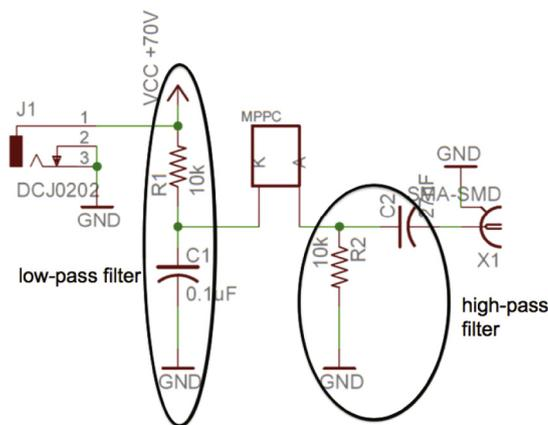
Fig. 1. A schematic diagram of the circuit used to read out the SiPMs. The SiPM is labeled as MPPC in the diagram.
