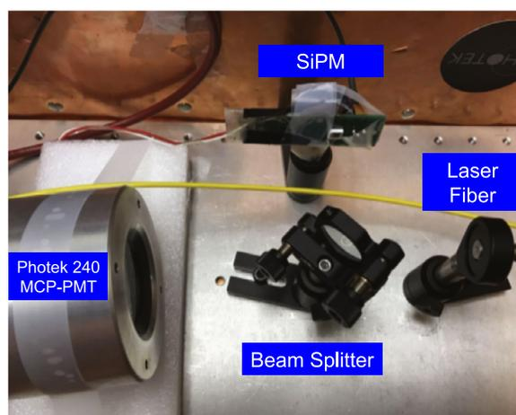
Fig. 2. Photograph of the Laser-based SiPM timing measurement setup.
