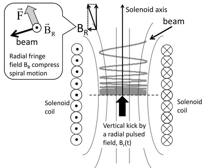
Fig. 1. Schematic magnetic force lines, muon orbit and radial magnetic field component.
