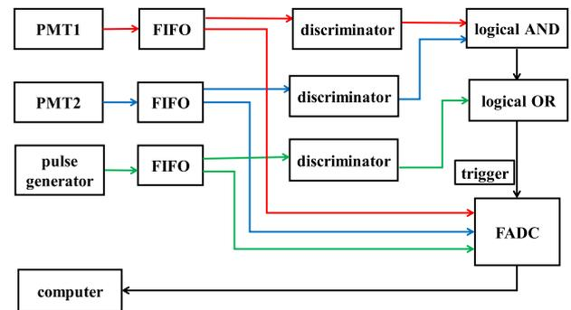
**Fig. 3.** The flow scheme of the data acquisition (DAQ) system. The duplicate signals are generated by linear fan-in/fan-out (FIFO) modules from the two PMTs, as well as the periodic pulse generator. One is fed into the discriminator, and the other is read out by a flash analog-to-digital converter (FADC). The DAQ triggers are provided by the coincident signals of the two PMTs and by the periodic signals from the pulse generator.
