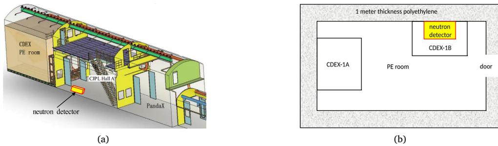
**Fig. 1.** (Color online) The structure of the China Jinping Underground Laboratory and the location of the neutron detector. (a) The position of the Hall A and the polyethylene (PE) room; (b) The structure of the PE room.
