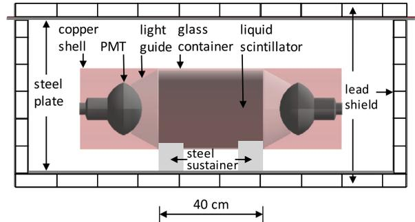
**Fig. 2.** (Color online) The schematic diagram of the liquid scintillator detector. The liquid scintillator is EJ-335. The container for EJ-335 is a quartz glass cylinder with 30 cm diameter and 40 cm length. The copper shell is used for supporting and shielding. The detector is located in a lead castle with 5 cm thick walls. The top steel plate is used to hold the roof of the lead castle. The bottom one is used to support the detector with two steel sustainers.
