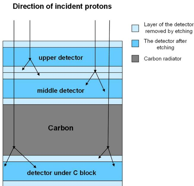
Fig. 2. Composition of the PADC stacks irradiated by high energy protons: target fragments are formed inside the material of the detector sheets and also inside the Carbon blocks. If the range is low, the tracks disappear after etching. The incident protons with high energy and low LET cannot produce tracks. The dimensions are not to scale.
