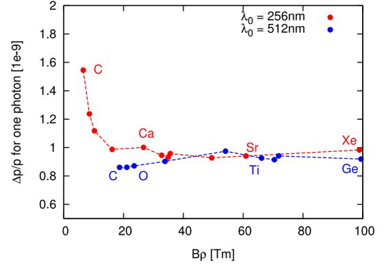
Fig. 1. Mean value of relative momentum kick for one scattering event, calculated for the  $2s_{1/2} \rightarrow 2p_{1/2}$  transition in Li-like ions. The transferred momentum stays nearly constant for different magnetic rigidities. Different dots represent different ions, which are partly marked by their element name.
