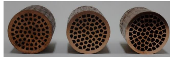
Fig. 1. UniPore samples with different porosities ( p = 0.32, 0.49, 0.58 ).
