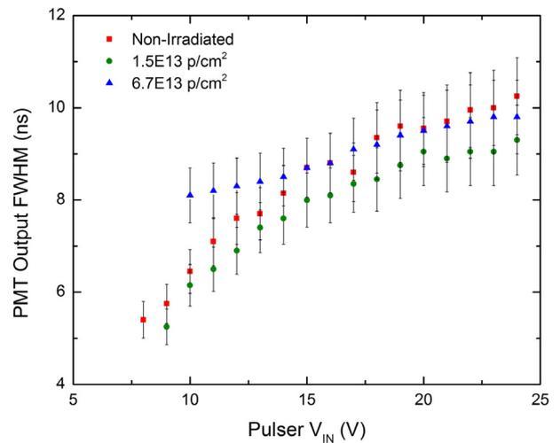
Fig. 4. Pulse width of the pulser before and after proton irradiation to fluences of  $1.5 \times 10^{13}$  and  $6.7 \times 10^{13}$  800-MeV-p/cm<sup>2</sup>.
