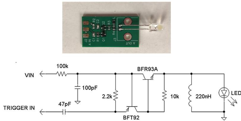
Fig. 1. The pulser circuit and board.
