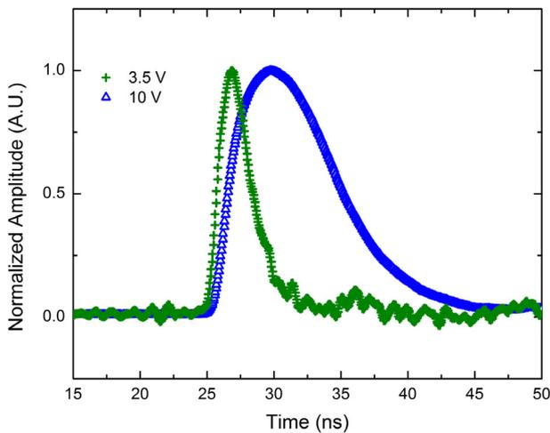
Fig. 3. Output pulse width of a non-irradiated pulser board at  $V_{IN} = 3.5$  V and  $V_{IN} = 10$  V.
