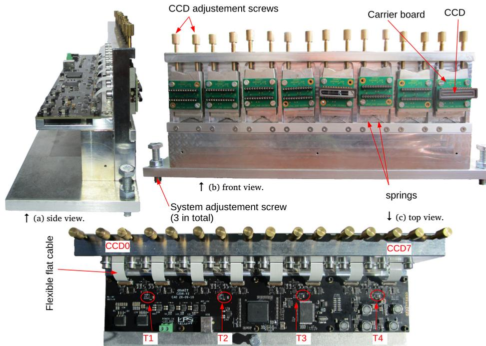
**Fig. 1.** Picture of the readout electronics mounted on its mechanical support. The electronic system is composed of two parts: the front-end composed of 8 carrier boards, each holding a CCD, and the back-end with the control and readout circuits. The boards are mounted on a mechanical support system equipped with adjustment screws to allow the adjustment of each CCD carrier board position. The four thermal sensors implemented on the board are indicated (T1 to T4).
