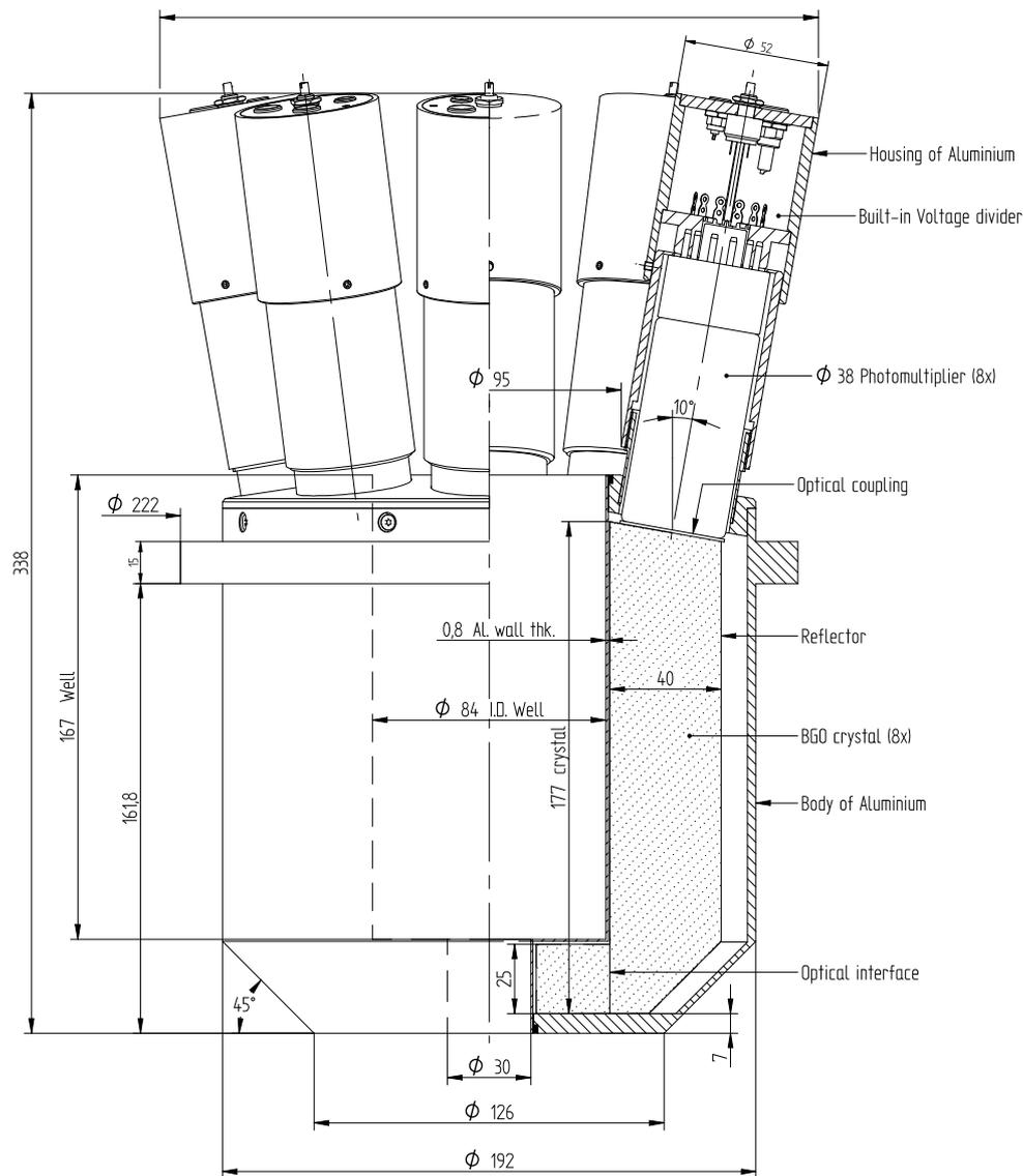
Fig. 1. The original design drawing for our Compton suppression system. The thickness of BGO hollow cylinder is 40 mm, the entrance window diameter is 30 mm and the HPGe detector diameter is 84 mm.
