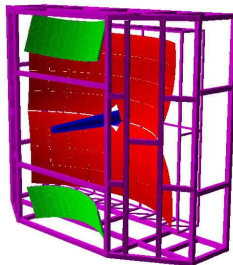
**Fig. 2.** Design of the CBM-RICH detector. Beside a  $\text{CO}_2$ -gaseous radiator it consists of a spherical mirror system and MAPMTs as photon detectors. The detector is separated into two halves above and below the beam pipe.
