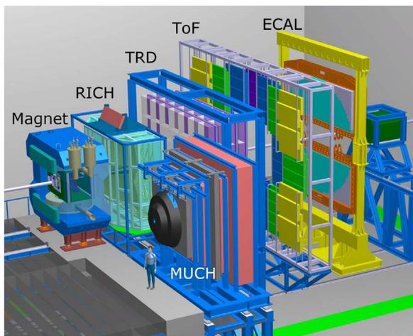
**Fig. 1.** Design of the CBM experiment. The tracking system STS is located inside the dipole magnet. The RICH detector is located directly after the magnet and before the other sub-detectors: TRD, TOF, and ECAL. The muon identification detector (MUCH) is shown in parking position.
