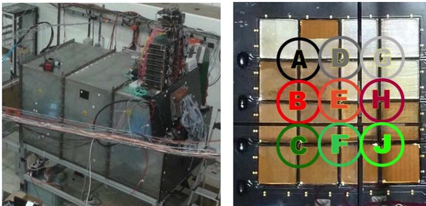
**Fig. 2.** Left: Photograph of the CBM-RICH prototype. Right: photograph of the PMT plane used during beam time at CERN-PS in 2014. Letters indicate tested ring positions.
