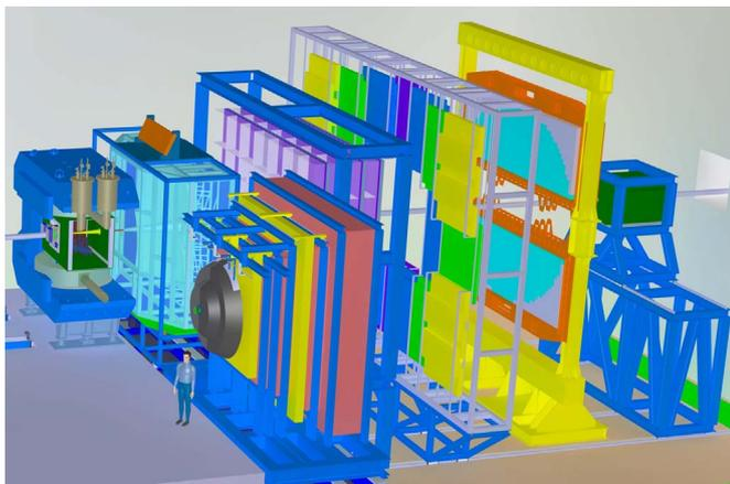
**Fig. 1.** Sketch of the CBM experimental setup. From left to right: STS tracking system inside a dipole magnet, RICH detector (Muons detector alongside), TRD detector, Time-of-flight wall (TOF), Electromagnetic CALorimeter (ECAL) and Projectile Spectator Detector (PSD).
