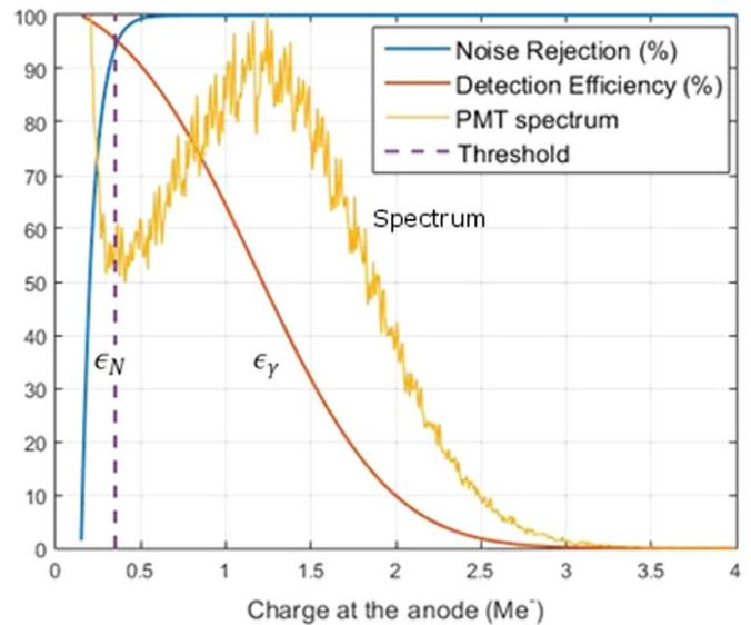
Fig. 2. Typical single photon spectrum, light signal detection efficiency ( $\epsilon_\gamma$ ) and dark counts rejection efficiency ( $\epsilon_N$ ) as a function of the signal amplitude. The dashed line shows the trigger threshold.
