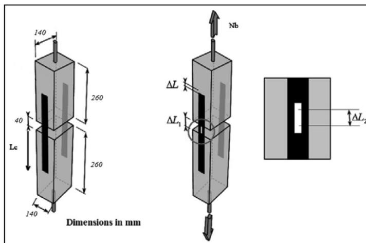
(a) Test principle of the double lap shear test
