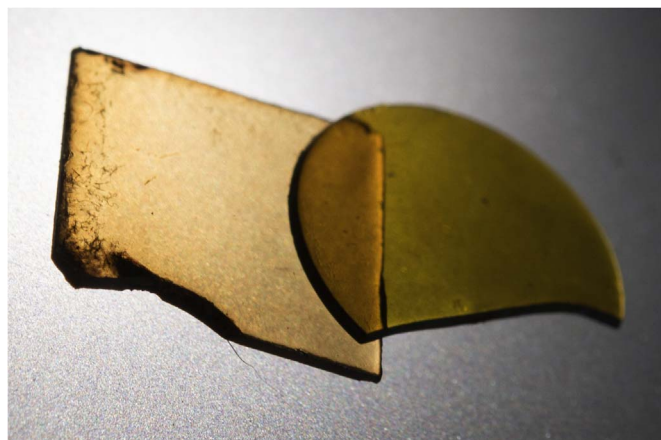
Fig. 1. Two semiconducting LISe crystals ( \sim 7 \text{ mm} largest dimension).
