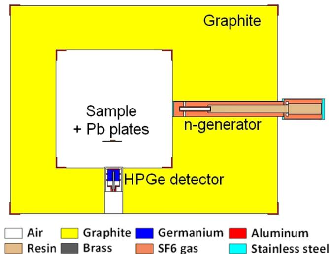
Fig. 2. MCNP model of the U and Pu samples measurements in REGAIN.
