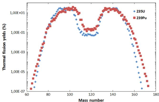
Fig. 1. Distribution of the cumulative thermal fission yields (fraction of fission fragment produced directly and via decay of precursors par 100 fissions induced by thermal neutrons) as a function of mass number, from JEFF3.1 database.
