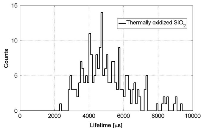
**Fig. 1.** A histogram of the lifetime data measured from a high-resistivity MCz-Si wafer oxidized at 1100 °C for 30 min resulting in 25 nm thick SiO<sub>2</sub>. During the PCD measurement both surfaces were Corona charged to +600  $\mu$ C charge in order to provide a field effect preventing the diffusing laser induced electrons to recombine into the surface states.
