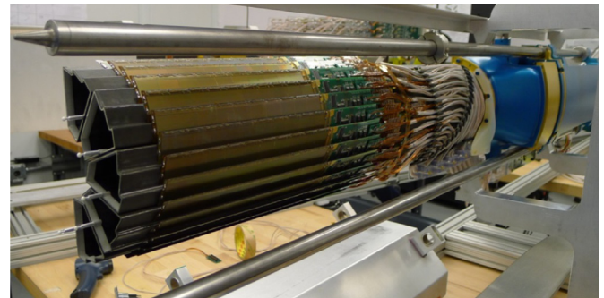
Fig. 2. PXL half-detector: 5 sectors mounted in dovetail slots on the carbon fiber support and connected to the insertion mechanics.
