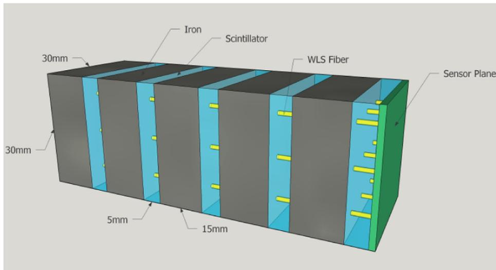
**Fig. 1.** Schematic of the ultra-compact module that is being developed by SCENTT. The module corresponds to a  $4 X_0$  sampling and a transverse granularity of  $3 \times 3 \text{ cm}^2$  (9 fibers per module).
