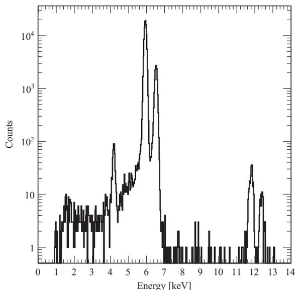
Fig. 1. Energy spectrum of  $^{55}\text{Fe}$  taken at 234 K with the SDD equipped with the silicon nitride window. The FWHM energy resolution is 141 eV for the 5.9 keV peak.
