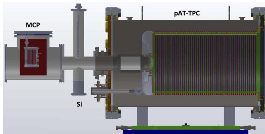
**Fig. 2.** Diagram of the MCP and the TPC. The chamber between them (labeled "Si") contains a Si detector that can be moved into the beam for tuning purposes.
