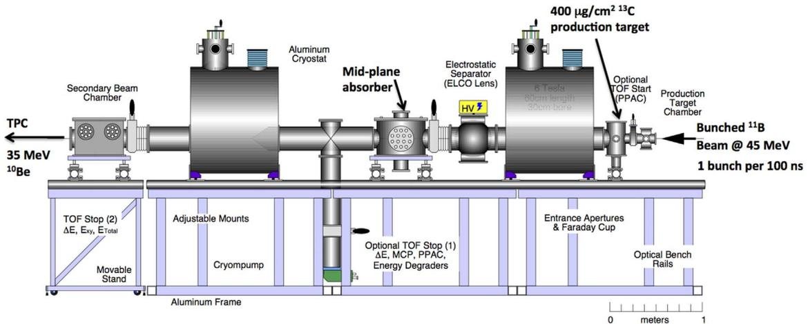
**Fig. 1.** *TwinSol* setup for  $^{10}\text{Be}$  beam production. The locations of the chambers containing the production target ( $^{13}\text{C}$ ,  $400\ \mu\text{g}/\text{cm}^2$ ) and mid-plane absorber ( $10\ \mu\text{m}$  Mylar) are indicated.
