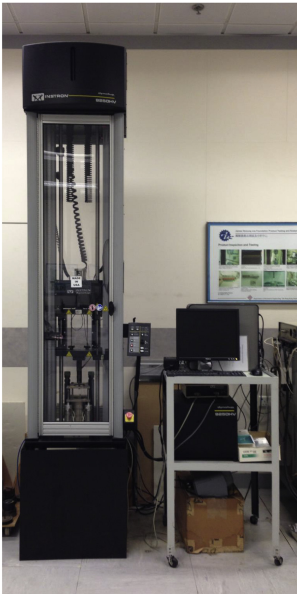
Fig. 1. Drop tower impact tester INSTRON Dynatup 9250 HV.
