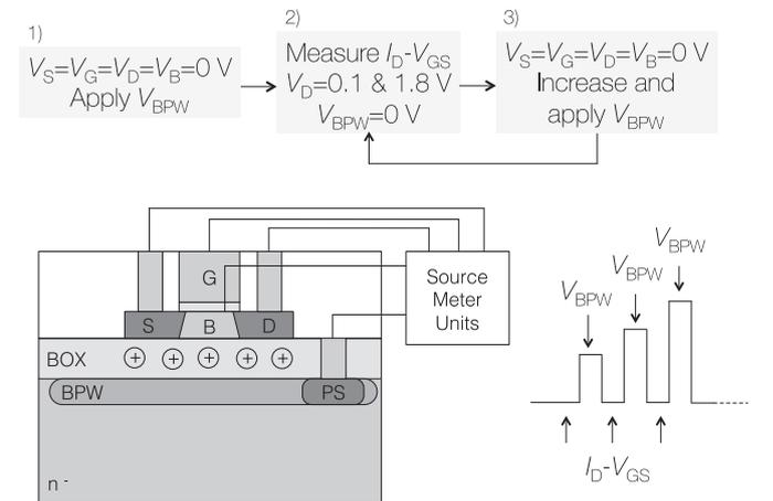
**Fig. 3.** Experimental setup and procedure for the measurement of the  $I_D$ – $V_{GS}$  characteristics and  $V_{BPW}$  pulses. (1) High-voltage pulses of  $V_{BPW}$  are applied to the BPW with the source, gate, and drain fixed at 0 V for FN tunneling between the BPW and the MOSFET through the BOX. (2) Measurement of the  $I_D$ – $V_{GS}$  characteristics with  $V_D = 1.8$  V to evaluate  $V_{th}$  and  $I_{leak}$ . (3) Iteration of (1) and (2) up to  $V_{BPW} = 150$  V.
