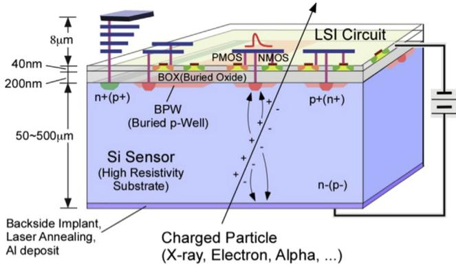
**Fig. 1.** Cross section of the SOI monolithic pixel detector. The readout circuit is processed on the top SOI layer. The buried oxide layer (BOX) is under the SOI layer. The buried p-well (BPW) is created under the BOX to suppress the back-gate effect. The voltage to the BPW can be supplied through the p<sup>+</sup> implant (PS). The thickness of silicon sensor under the BOX depends on application [9].
