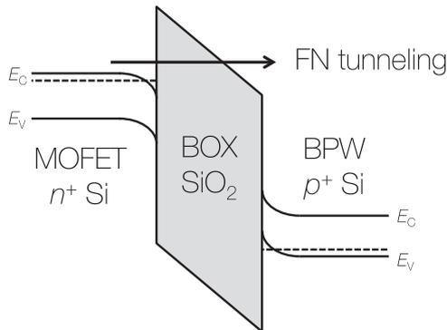
**Fig. 2.** Fowler–Nordheim tunneling. Electrons tunnel through the triangular potential of Si–SiO<sub>2</sub> junction. FN tunneling occurs at a high electric field of more than 0.5 GV/m.
