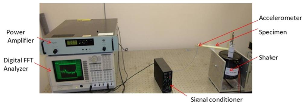
Fig. 2. Experimental setup.
