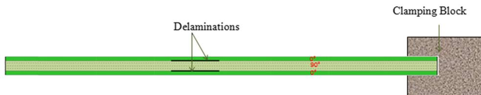
Fig. 1. Composite specimen with delamination.
