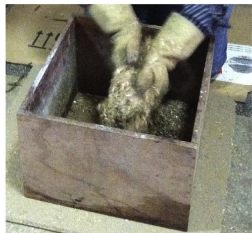
Fig. 2. Mixing procedure of short glass fibers and wood particles.
