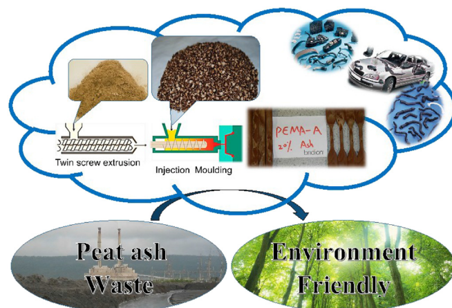
Fig. 1. Utilization of ash waste filled polymer composites for automobile applications.
