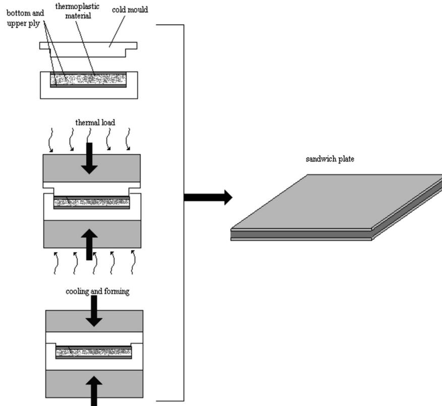
Fig. 1. Processes for aluminium-thermoplastic sandwich manufacturing: isothermal compression moulding.
