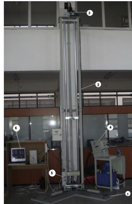
Fig. 2. Drop-weight test machine developed at Dumlupinar University: 1–L shape table, 2–weight drop tower, 3–lift engine, 4–control unit, 5–rebound breaking system, 6–data acquisition unit.
