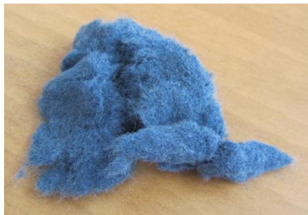
Fig. 1. Appearance of cotton flocks as received from differentiated waste collection of end-of-life jeans.
