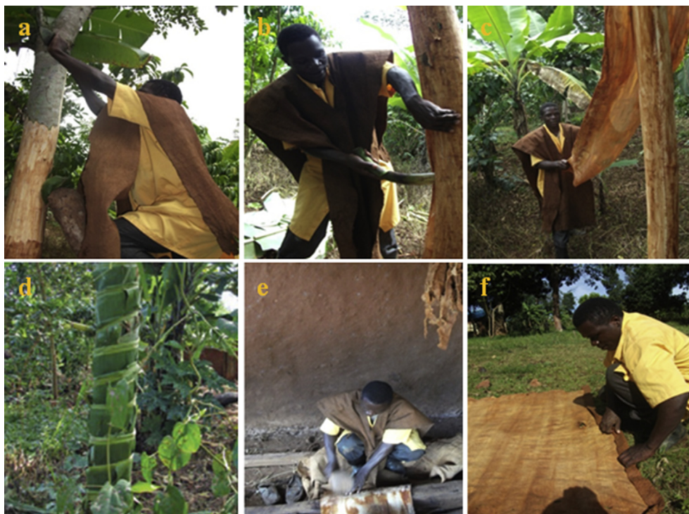
Fig. 1. Extraction of Bark cloth nonwoven natural fabric: (a) Scrapping of tree outer layer. (b) Use of local wedged tool to peel off the bark. (c) Peeling of the bark. (d) Covering of the tree stem for environmental sustainability. (e) Pummeling under the shade. (f) Sun drying of the non-woven fabric.
