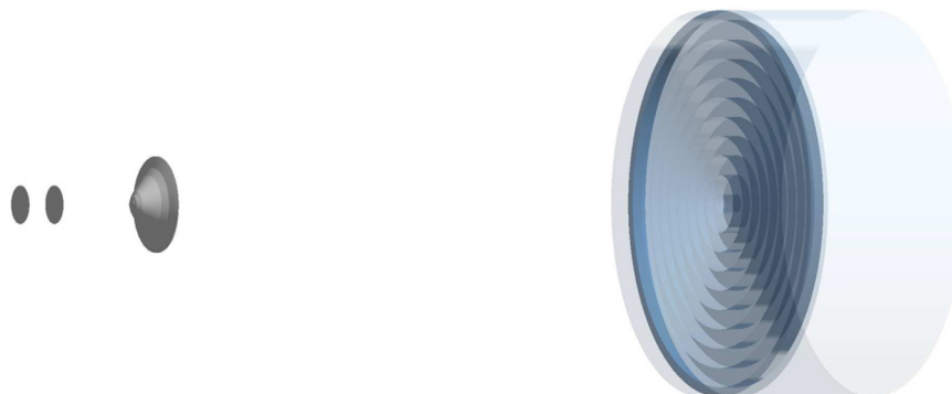
Fig. 1. Geant4 model of the most simple system geometry. From left to right: exit window, scattering foil, flattening foil, water phantom. The dimensions of foils were set unrealistically large in order to improve readability of the illustration. For the same reason also the number and dimensions of radial segments of the water phantom are for illustration purposes only, and do not reflect the actual system geometry.
