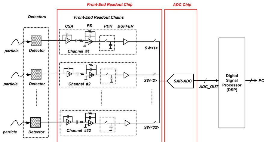
Fig. 2. Block diagram of typical 32-channel CZT detector PET imaging system.
