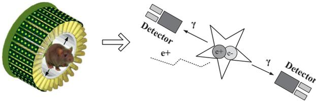
Fig. 1. Principle of PET imaging.
