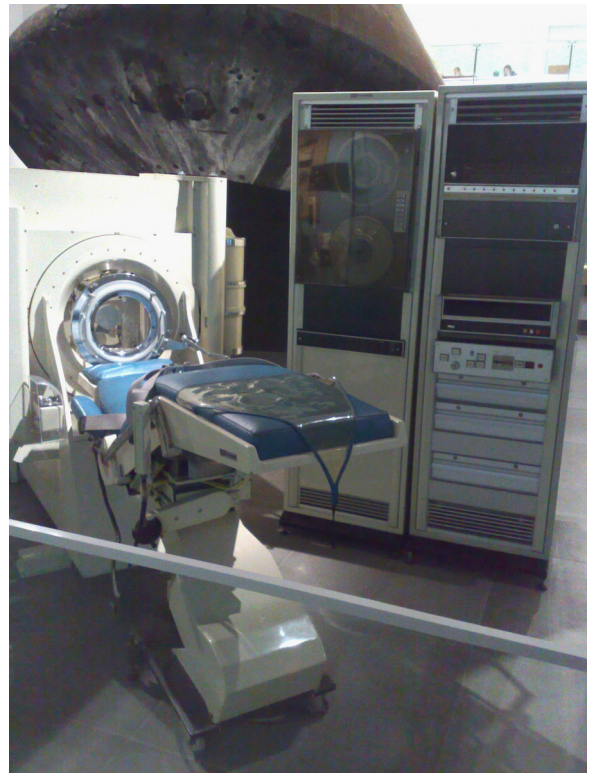
Fig. 1. The EMI Mark I scanner at the South Kensington Science Museum, London. The rubber cap used to separate the patient head from the water bag can be seen at the bore entrance. This water bag served to reduce the photon fluence at the periphery of the field of view (outside the skull’s margins), thus avoiding to saturate the very low dynamic range of the NaI-based detectors.
