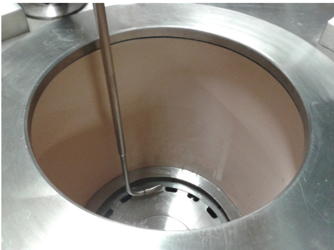
Fig. 1. Centrifugal drum and nozzle of a DSF.
