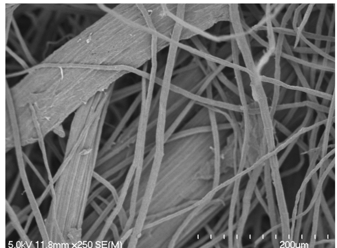
Fig. 2. SEM image of a fibre mat made from pulped harakeke using DSF.
