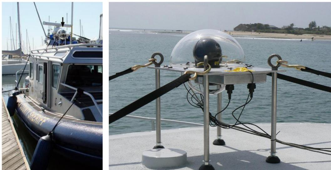
**Fig. 1.** Three-axis motion sensor and video camera mounted on the roof of a 33-ft police vessel (arrow on left) and a close-up of the package (right). The black spherical object is the gyro-stabilized video camera of a TASE inertial package [8]; the small box under the support plate on the right contains both a three-axis accelerometer and a magnetometer.
