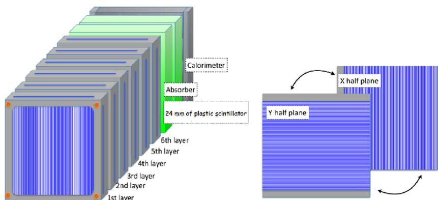
Fig. 1. Schematic picture of the dose profiler (left) and schematic picture of one of the tracker layers (right).
