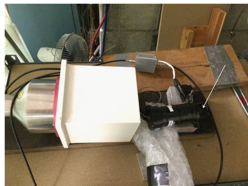
Fig. 2. The CLYC-7 scintillator (white arrow) shown with 51 mm super bialkali Hamamatsu PMT set-up at the Crocker Nuclear Laboratory experiment room.
