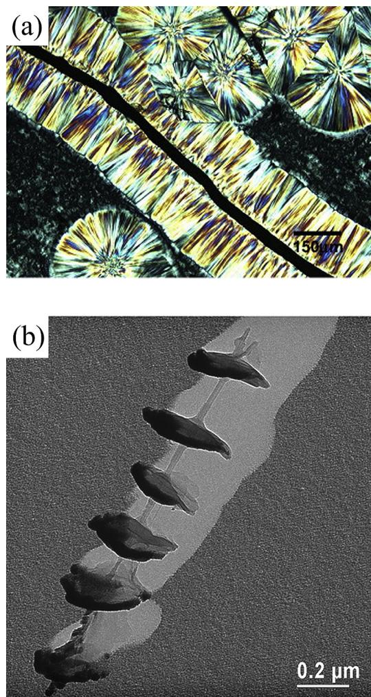
**Fig. 1.** TEM micrograph of CNT induced interfacial crystallization. (a) The transcrystallinity layer (TCL) [16]; (b) The nanohybrid shish-kebab (NHSK) structure [17].
