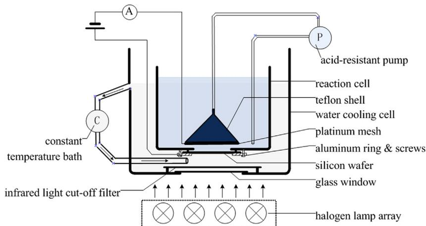
**Fig. 4.** Schematic diagram of the photoelectrochemical etching setup.
