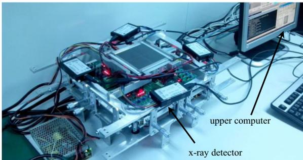
**Fig. 3.** Photograph of the  $2 \times 2$  FOT array coupled digital x-ray detector without the pixelated scintillator.
