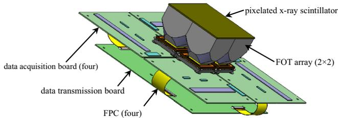
**Fig. 1.** Schematic representation of the  $2 \times 2$  FOT array-coupled digital x-ray detector.
