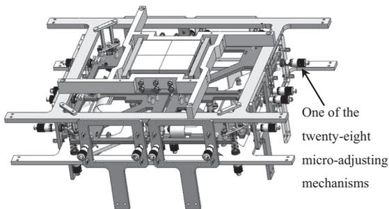
**Fig. 2.** Sketch of the six-dimensional adjustable coupling system between the FOT array and the four CMOS image sensors.
